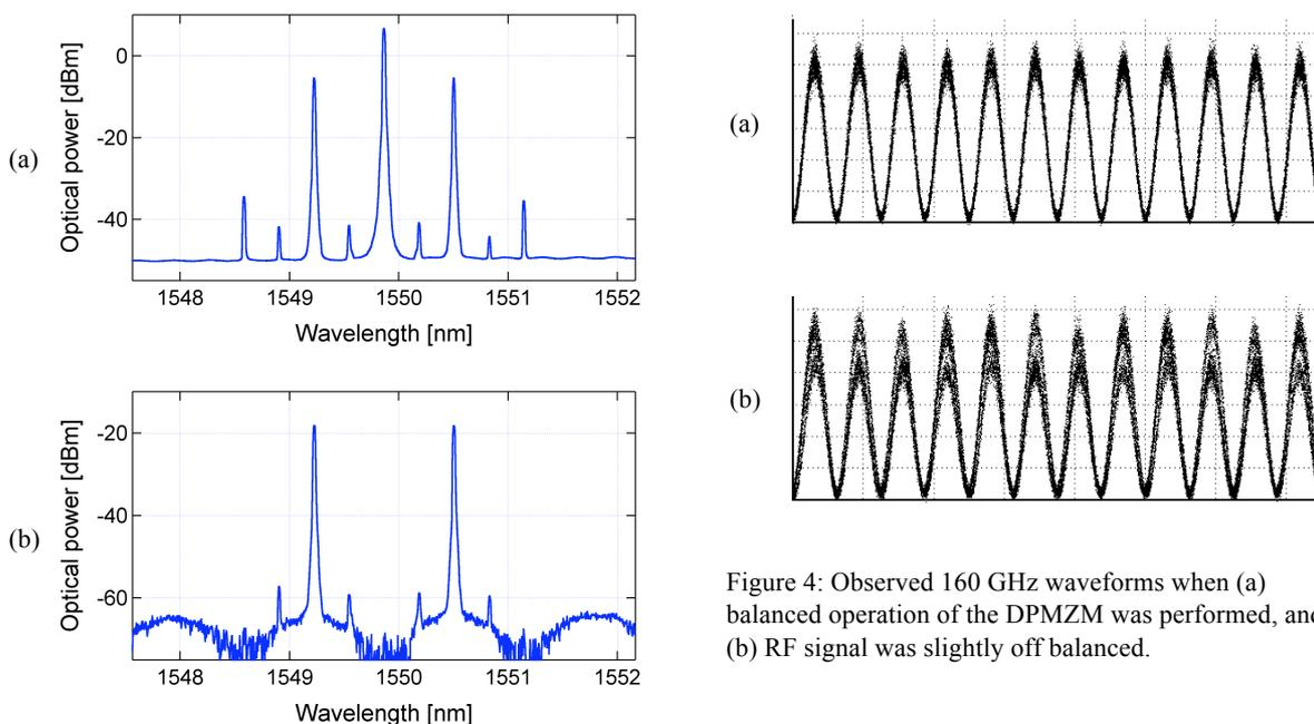
Figure 3: Observed optical spectra (a) without DI and OBRF, and (b) with DI and OBRF.
