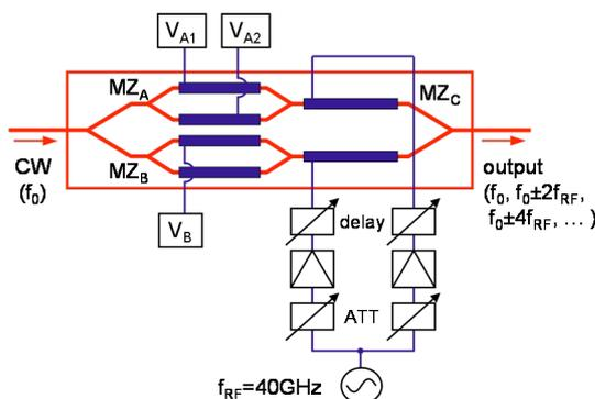
Figure 1: Schematic of DPMZM and driving circuit for highly balanced operation.  $V_{A1}$ ,  $V_{A2}$  and  $V_B$  are DC bias voltages
