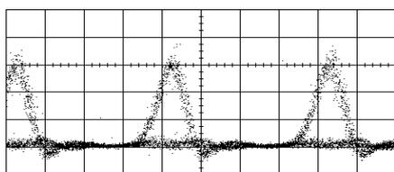
Fig. 5 Observed waveform of a demultiplexed 10 Gbit/s signal at 2,600 km.
