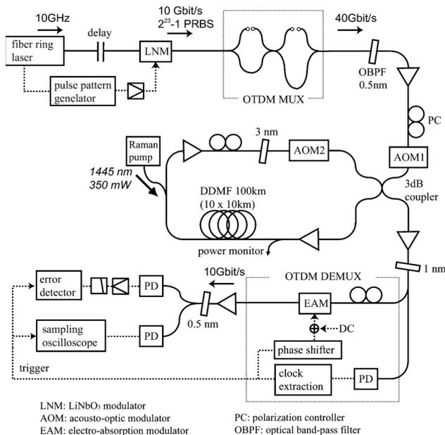
Fig. 3 Experimental setup.
