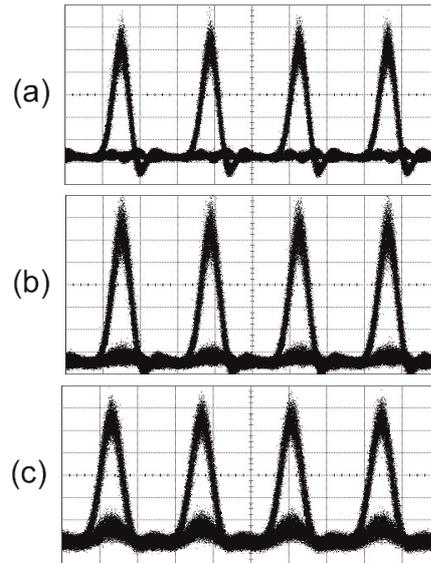
Fig. 3 Eye diagrams of the transmitted signals after 20 Gbit/s-to-10 Gbit/s OTDM DEMUX. (a) ch1 (1536.61 nm), (b) ch38 (1566.31 nm) and (c) ch75 (1597.19 nm).
