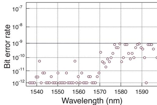
Fig. 4 Measured BER performances of 75 WDM channels.
