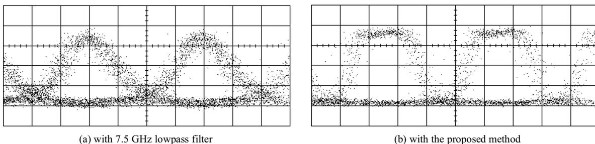
Fig. 2. Eye diagrams of the detected 10 Gb/s solitons at 12,000 km (25 ps/div).
