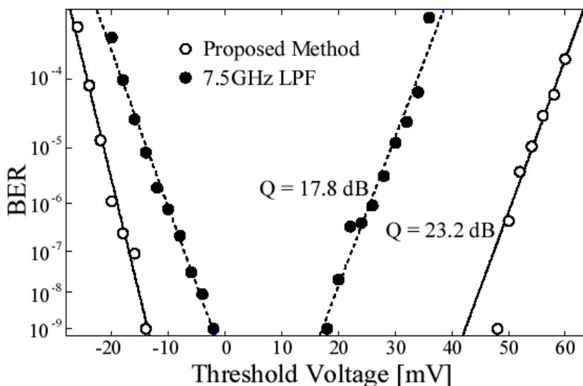
Fig. 3. Measured bit error rate while changing the threshold voltage with the detection time adjusted to maximize the amplitude margin in each case
