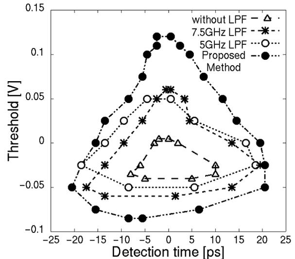
**Figure 4: Measured threshold and detection time of BER detector where BER is below  $10^{-7}$ .**
