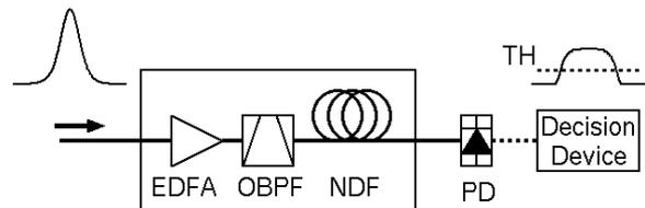
**Figure 2: Schematic diagram of the setup for phase margin improvement.**
