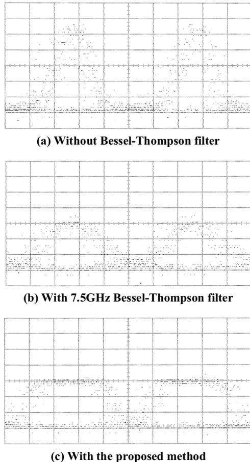
**Figure 3: Eye diagrams of the transmitted 10 Gbit/s soliton in a sliding frequency recirculating loop over 16,000 km (20 ps/div).**
