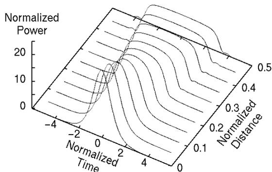
**Figure 1: Pulse shapes propagating along normal dispersion fiber with Kerr nonlinearity.**
