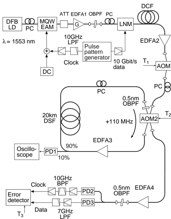
EAM : electroabsorption modulator, LNM : LiNbO<sub>3</sub> intensity modulator
