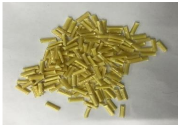
PA66 + Aramid fiber Fiber length: 7mm
