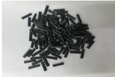
PA66 + Carbon fiber Fiber length: 9mm
