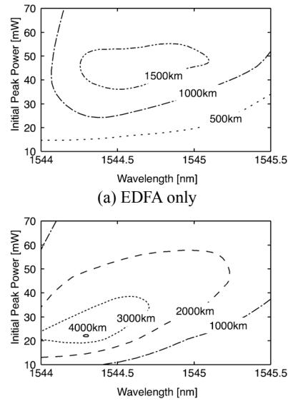
Fig. 2 Calculated transmission distance where  $Q = 6$  vs input peak power to the fiber and wavelength.
