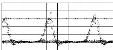
Fig. 5 Observed waveform of a demultiplexed 10 Gbit/s signal at 2,600 km.
