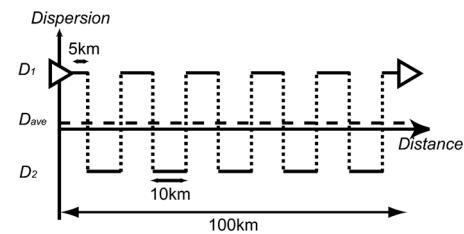
Fig. 1 Dispersion map of the dense dispersion managed fiber.
