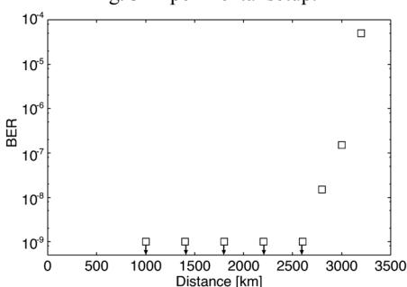
Fig. 4 BER versus transmission distance.
