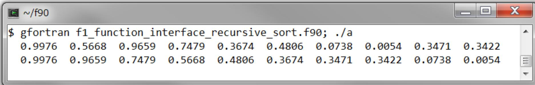
A terminal window titled '~ /f90' showing the compilation and execution of a Fortran program. The command executed is '\$ gfortran f1\_function\_interface\_recursive\_sort.f90; ./a'. The output consists of two lines of ten floating-point numbers each, representing the sorted array. The first line is the original array, and the second line is the sorted array.
