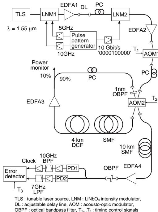
The timing jitter was estimated by measuring the BER versus deviation of decision time  $t_d$  [ps] of the error detector/13/. In this paper, we assume that (1) the waveform of transmitted DM soliton is constant, (2) no noise and no amplitude fluctuation are included in the DM soliton, and (3) the timing jitter obeys a Gaussian distribution with the standard deviation of  $\sigma$  [ps]. Under these assumptions, the BER of 10-Gbit/s 0000100000 data can be obtained by the following equation
