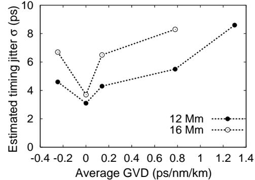
Figure 3 shows the estimated timing jitter versus  $D_{ave}$  of the transmission fiber at 12 Mm and 16 Mm. The figure clearly shows that the jitter is minimized when  $D_{ave}$  is zero.
