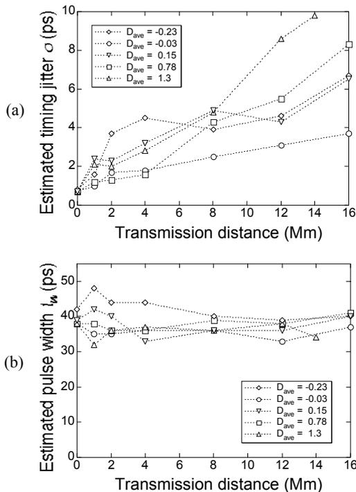
The estimated timing jitter obtained when  $D_{ave} = -0.23$  ps/nm/km before 4 Mm was larger than those obtained in other  $D_{ave}$ 's at the same transmission distance. In the case where the pulses include noise or amplitude fluctuation, the estimated  $\sigma$  may be described as follows
