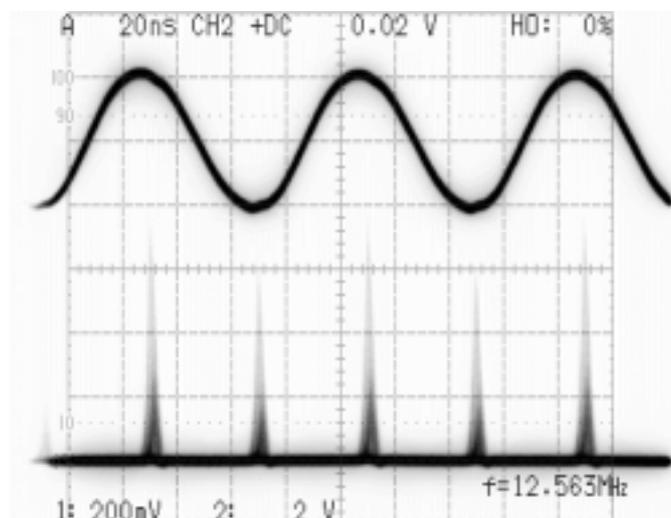
Fig. 5 Generated optical pulses by rational mode locking of the fiber loop for loop length adjustment.
