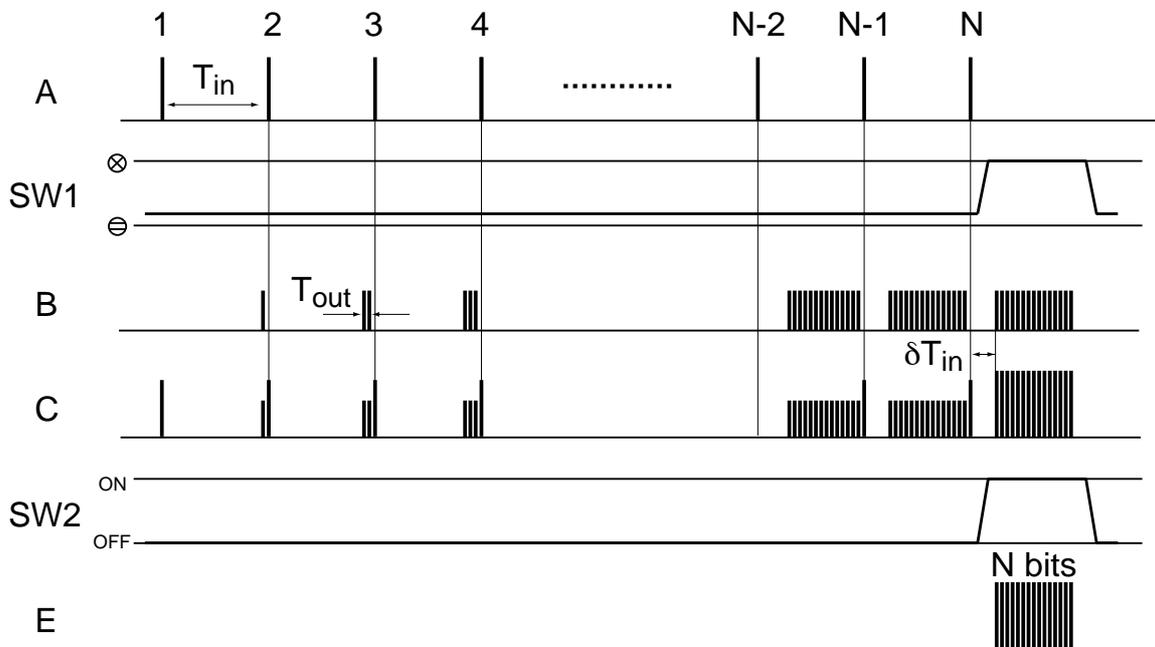
Fig. 2 Timing chart of compression operation of an N-bit optical packet.
