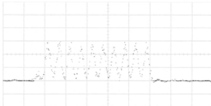
Fig. 7 Observed waveform of the compressed 10 bit packet (400 ps/div).
