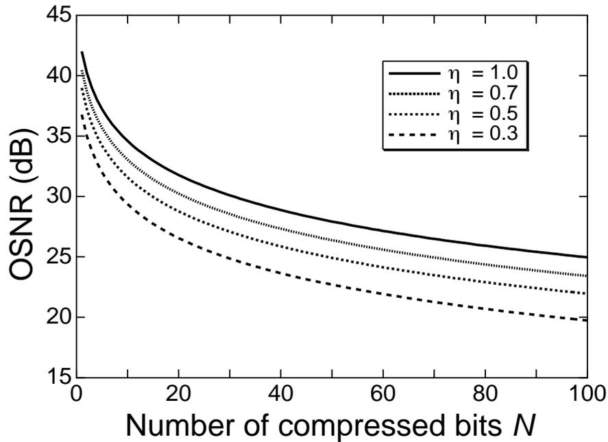
Fig. 3 Calculated optical signal-to-noise ratio of output packet with 1 nm bandwidth versus number of compressed bits  $N$ .
