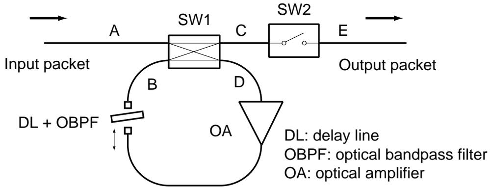
Fig. 1 The schematic view of the proposed optical packet compressor.
